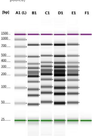
**Figure 6. BioFluidica cfDNA chips capture low molecular weight DNA.** As proof of concept, low molecular weight (LMW) DNA ladder using various conditions was run through the cfDNA microfluidic chip and eluted following isolation. LMW DNA was recovered demonstrating the efficacy of the Liquid Scan to isolate cfDNA.
