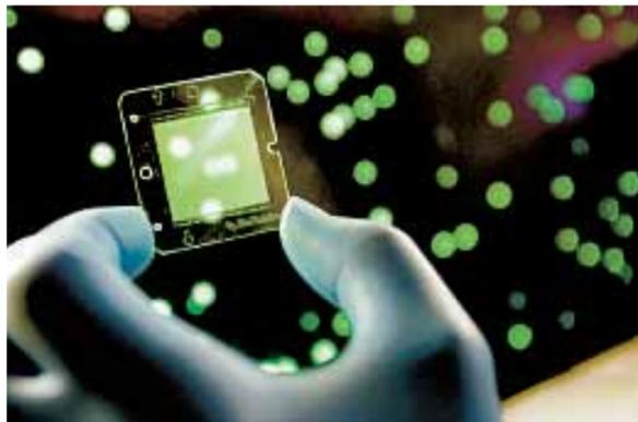
A microfluidic chip, recently developed by BioFluidica to capture abnormal cells, is held up to a computer image of breast cancer cells that were isolated by the chip.
