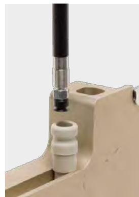
CO-RE Lid Tool on its Park Position on the Waste Station
