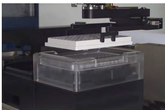
The iSWAP in action to load a filter plate to the CVS
