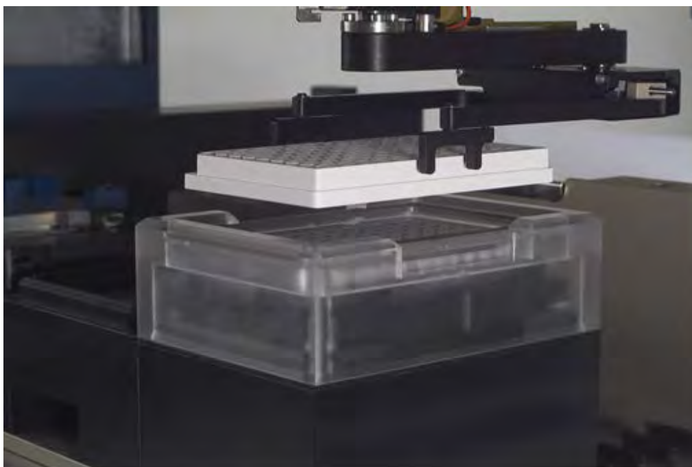
iSWAP Robotic Hand at work Transporting Microplates to the CVS
