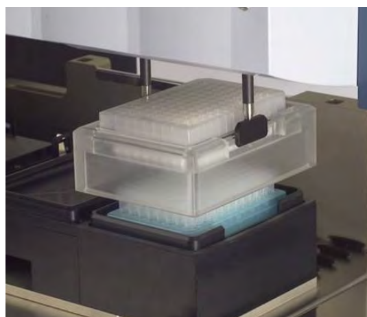
CO-RE Gripper on 1000µl-Pipetting Channels
