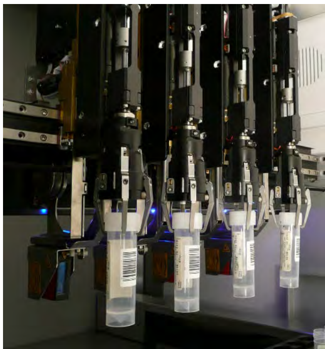
Four Tube Twister Channels holding tubes
