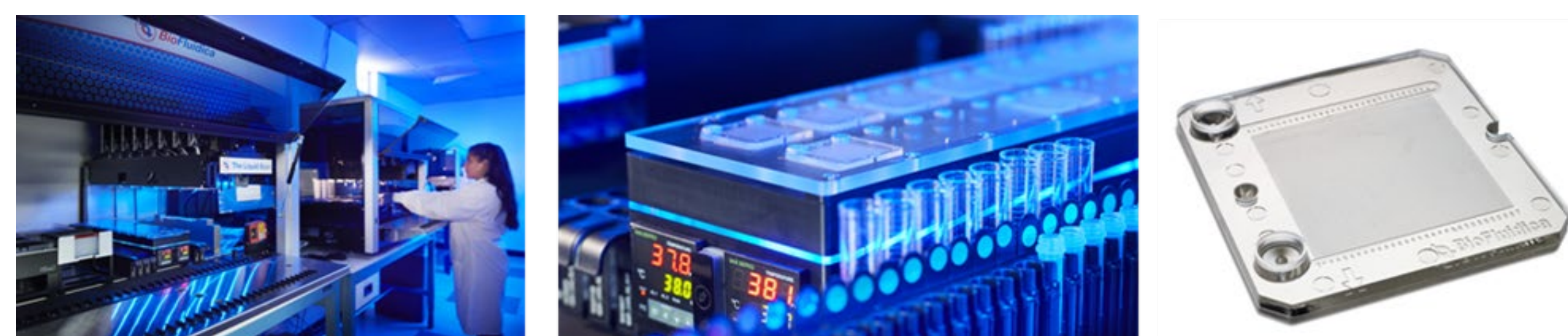
Figure. LiquidScan instrumentation has "Hamilton Inside" (First image). The blood sample tube is placed on the robot, and the operator can walk away. Chips (Third image) are housed on the LiquidScan module (second image), up to eight per run. Whole blood is introduced directly from the sample tube into the biomarker isolation chip. Blood is slowly injected (pushed) into one port on the chip and simultaneously withdrawn on the other port (a push-and-pull no loss system). The robotic system is scalable for fully automated processing. In this study, the microfluidic chip is surfaced with antibodies to specifically capture CTCs from whole blood.
