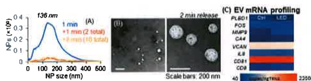
Fig. 3 EVs affinity-enrichment (anti-CD8 mAbs). The EVs were enriched from MOLT-3 conditioned media and released by LED exposure from the EV enrichment microfluidic device. The released EVs were subjected to NTA (A), TEM (B), and ddPCR (C). The ddPCR was carried out on 8 genes. Among them, five genes ( PLBD1 , FOS , MMP9 , CA4 and VCAN ) are known to be dysregulated as a result of AIS event. See Table S3 (ESI†) for the sequences of the primers used for the ddPCR.
